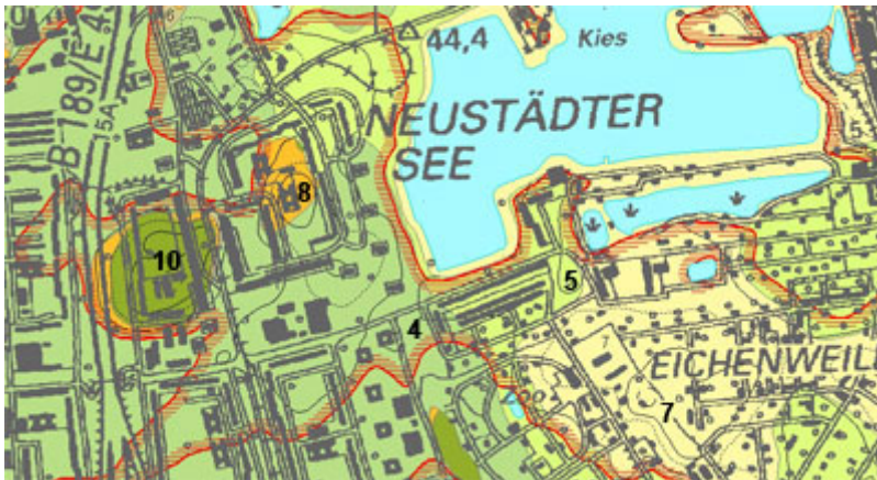
Figure 7. Engineering geological map of the city of Magdeburg (Annotation: distribution of anthropogenic deposits with thickness contours. See Figure 5 for explanation of the numbers).
